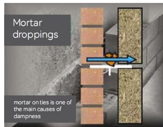
Fig3—Mortar dropping causing dampness
